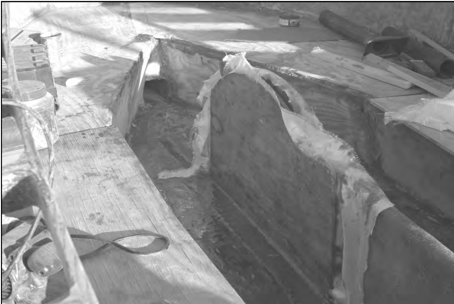
Earlier in the rehab process Charlie Smith was working on the center board trunk. He's probably still got a few hours of work ahead of him; but he's moving forward.
