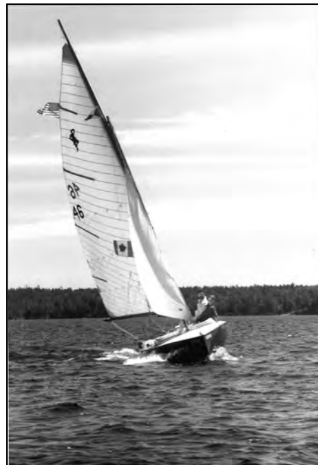
In Parry Sound, standard Highlander mainsail set as Solent lugsail; storm jib.
