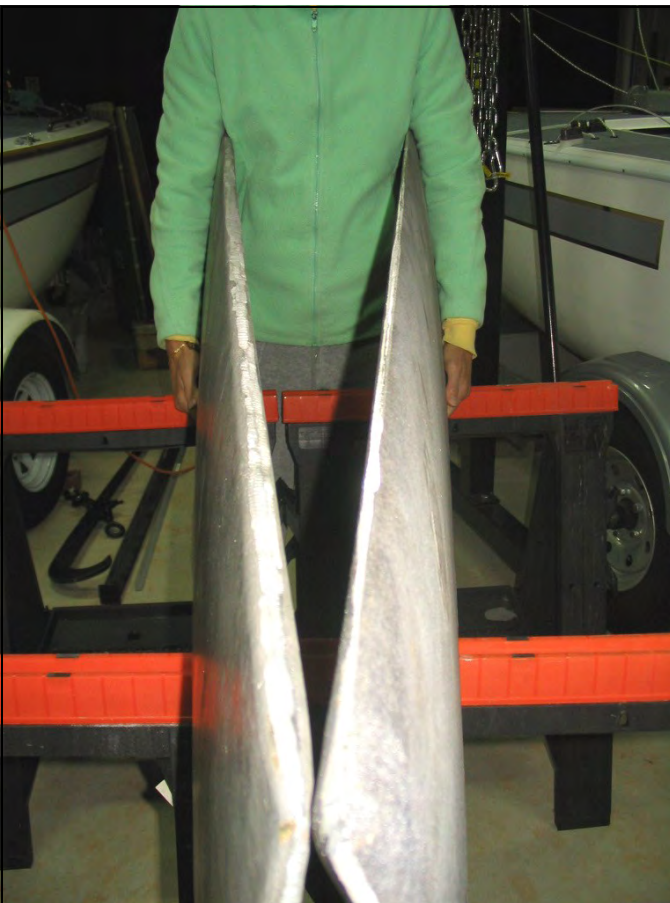
Blunt, old, leading edge on left, new slim profile on right.
